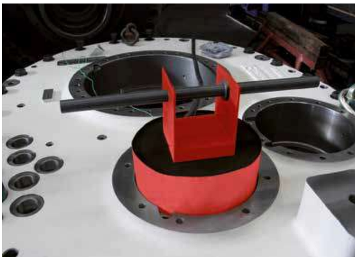
Heating bores in housings For mounting bearings and pins (including in frames and gearboxes).
