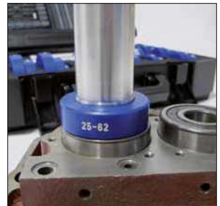
Collets are engraved and marked clearly
